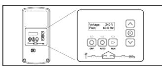
The RDC2 controller provides integrated control for the generator set, Kohler<sup>®</sup> Model RXT transfer switch, programmable interface module (PIM), and load shed kit.
