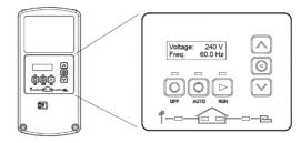
The RDC2 controller provides integrated control for the generator set, Kohler $^{\odot}$  Model RXT transfer switch, programmable interface module (PIM), and load shed kit.
